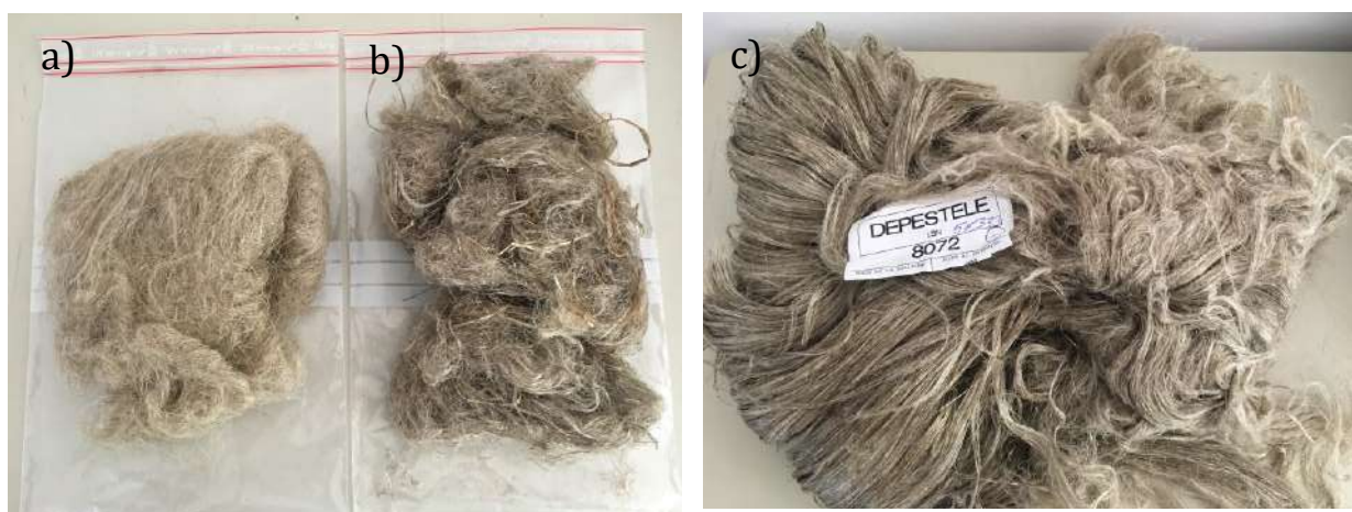
Figure 1 : Pictures of the material provided by DEPESTELE : a) High quality tows b) Tows with shives c) High quality fibers 8072es
