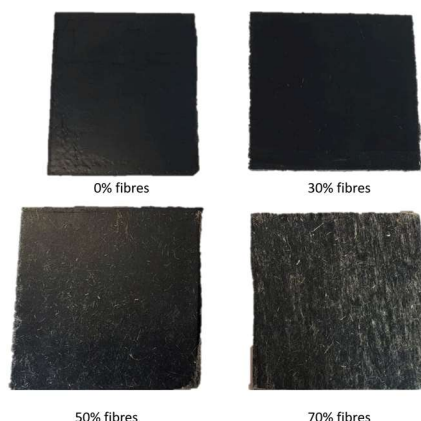
Figure 3 – Plates obtained with different PLA-Flax ratios
