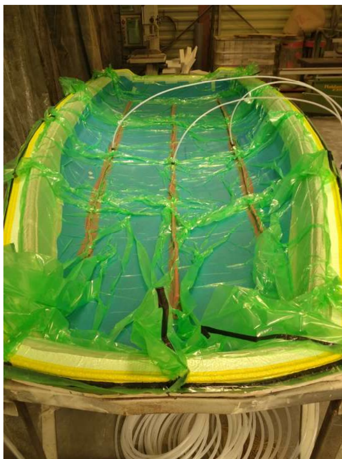
Placement of the vacuum tank and injection bars
