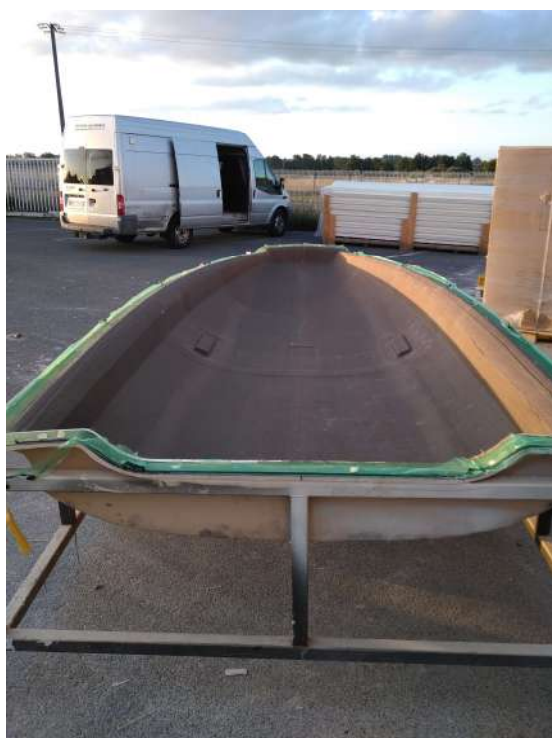
Demoulding of the hull
