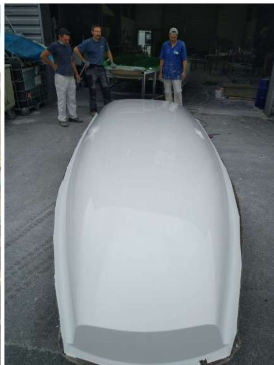
Demoulding of the hull
