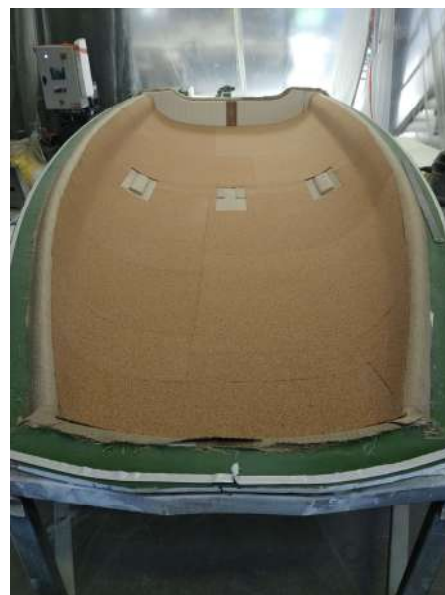
Draping of cork core material
