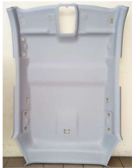
Operation to cut the thermoformed headliner in a final part
