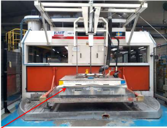
Headliner in position on the cutting support water jet
