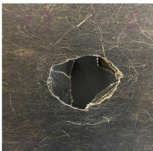
Fig 6. Appearance of NNW samples after impact test
