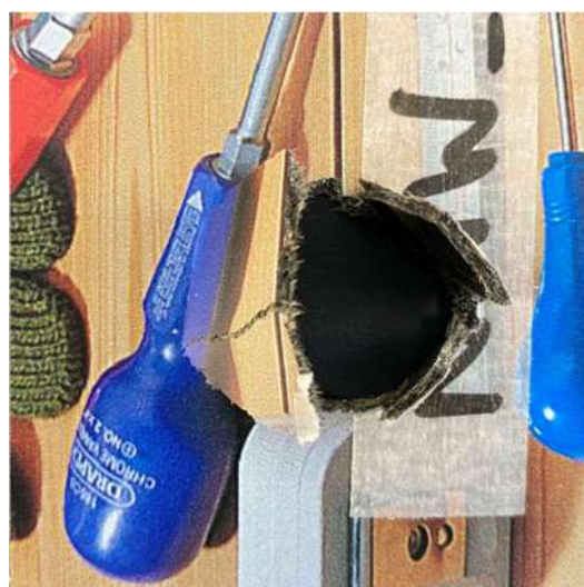
Fig 6. Appearance of NNW samples after impact test
