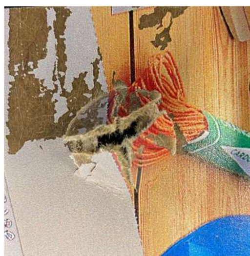
Fig 5. Appearance of CNW samples after impact test
