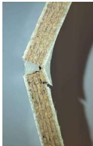
Figure 5 : faciès de rupture
