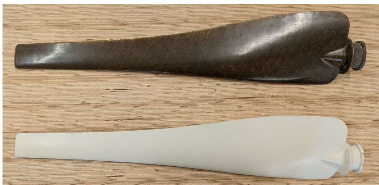
Figure 5. The flax-epoxy composite prototype blade, sitting in relation to the conventional glass/nylon blade.
