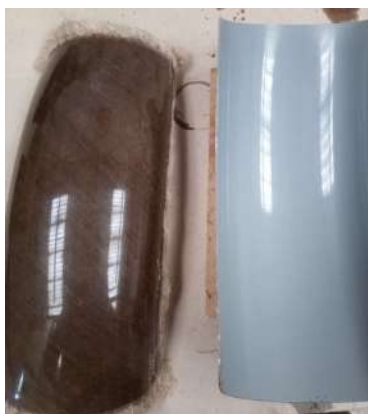
Figure 2. A preliminary successful trial hand lay-up trial on the mould tool surface.
