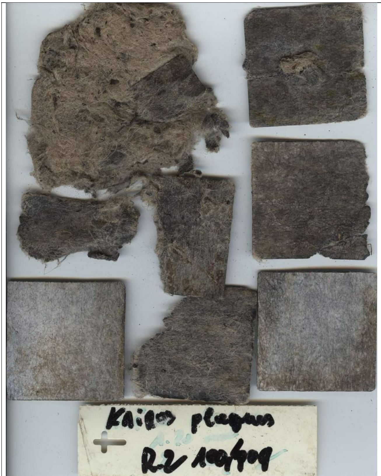
Repetition 2 – Filamentous residues and a few slightly disintegrated platelets - 18.15 grams for 100.40 grams initial weight
